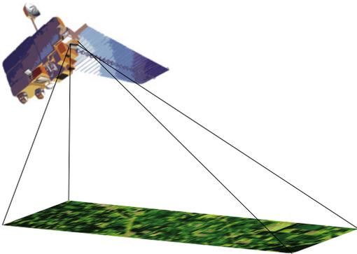
The MODIS instrument aboard NASA's Terra satellite measures average vegetation cover across pixels of 250 m<sup>2</sup>. Though this resolution could miss variation in conditions within that area, these measurements can still be used to accurately estimate crop yields.
